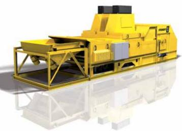
All STEINERT KSS machines are equipped with active valve control for up to 30 % lower compressed air consumption. The required air blast pressure and the number of the controlled compressed-air valves can be optimally adjusted. The nozzle bar is particularly exact thanks to its grid of pairs of nozzles spaced at 12.5 mm intervals. Your advantages: Optimised separation and reduced operating costs.
