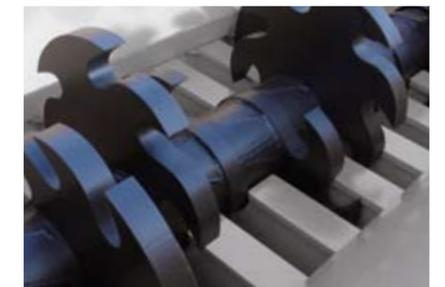
The knives are solidly welded onto the shafts; there are no bolts, bearings or adjustable parts anywhere in the cutting area, reducing servicing requirements.
