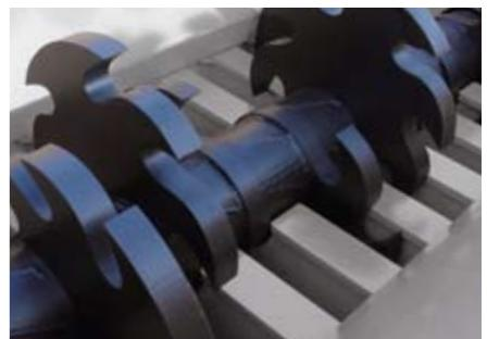
The knives are solidly welded onto the shafts; there are no bolts, bearings or adjustable parts anywhere in the cutting area, reducing servicing requirements.
